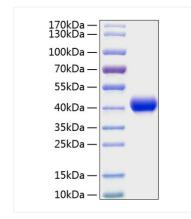
Recombinant Mouse CXCL16/SR-PSOX Protein was determined by SDS-PAGE with Coomassie Blue, showing a band at 38-45kDa.
