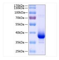
Recombinant Human TNFRSF12A/TWEAKR/CD266 Protein was determined by SDS-PAGE with Coomassie Blue, showing a band at 35-45 kDa.
