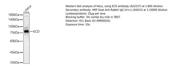
Western blot analysis of various lysates, using ECD antibody (A22237) at 1:800 dilution. Secondary antibody MRP Goat Anti-Rabbit IgG (H+L) (AS014) at 1:10000 dilution. Lysates/proteins, 25µg per lane. Blocking Differ 3% nonfat dry milk in TBST.
