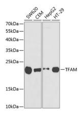
Western blot analysis of extracts of various cell lines, using TFAM antibody (A1926) at 1:1000 dilution. Secondary antibody: HRP Goat Anti-Rabbit IgG (H+L) (AS014) at 1:10000 dilution. Lysates/proteins:  $25\mu g$  per lane.
