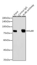
Immunoprecipitation analysis of 300  $\mu$ g extracts of HeLa cells using 3  $\mu$ g Ku80 antibody (A12338). Western blot was performed from the immunoprecipitate using Ku80 antibody (A12338) at a dilution of 1:1000.
