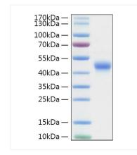
Recombinant Mouse TNFRSF4/OX40/CD134 Protein was determined by SDS-PAGE with Coomassie Blue, showing a band at 40-55kDa.
