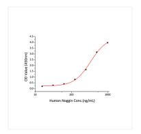
Immobilized recombinant Human BMP4 at 0.5  $\mu$ g/mL (100  $\mu$ L/well) can bind Noggin with a linear range of 16-314 ng/mL.
