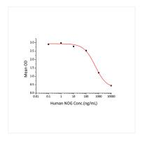
Recombinant human NOG inhibits BMP-4-induced alkaline phosphatase production by ATDC5 mouse chondrogenic cells.The ED $_{50}$  for this effect is 0.26-1.06  $\mu$ g/mL in the presence of 50 ng/mL of Recombinant Human BMP-4.
