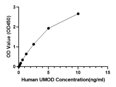
The standard curves are provided for demonstration only. A standard curve should be generated for each set of UMOD assayed.
