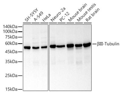
Western blot analysis of various lysates, using  $\beta$ III-Tubulin Rabbit pAb (A11933) at 1:500 dilution.
