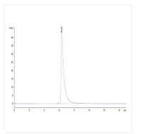
The purity of SARS-COV-2 Spike S Trimer is greater than 95% as determined by SEC-HPLC.
