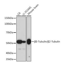
Western blot analysis of various lysates using  $\beta$ II-Tubulin/ $\beta$ 2-Tubulin Rabbit mAb (A4798) at 1:1000 dilution.
