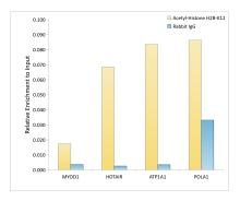
Chromatin immunoprecipitation analysis of extracts of HeLa cells, using Acetyl-Histone H2B-K12 antibody (A15619) and rabbit IgG.The amount of immunoprecipitated DNA was checked by quantitative PCR. Histogram was constructed by the ratios of the immunoprecipitated DNA to the input.
