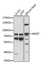
Western blot analysis of various lysates using ABCB7 Rabbit pAb (A14699) at 1:1000 dilution. Secondary antibody: HRP Goat Anti-Rabbit IgG (H+L) (AS014) at 1:10000 dilution.
