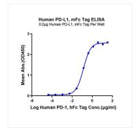
Immobilized Human PD-L1, mFc Tag at 2µg/ml (100µl/Well) on the plate. Dose response curve for Human PD-1, hFc Tag with the  $EC_{s0}$  of 0.13µg/ml determined by ELISA.
