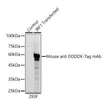
Western blot analysis of lysates from 293F cells transfected with IRF1-Flag protein , using HRP-conjugated Mouse anti DDDDK-Tag mAb (AE024) at 1:5000 dilution.
